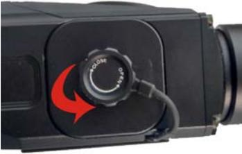
Fig. 6 open battery cover
