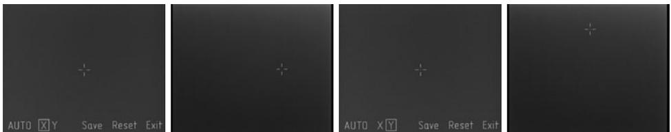
**To cancel** the dead pixels removal press and hold button M for more than 2 sec with the option "Reset" selected. The display shows the confirmation request.
