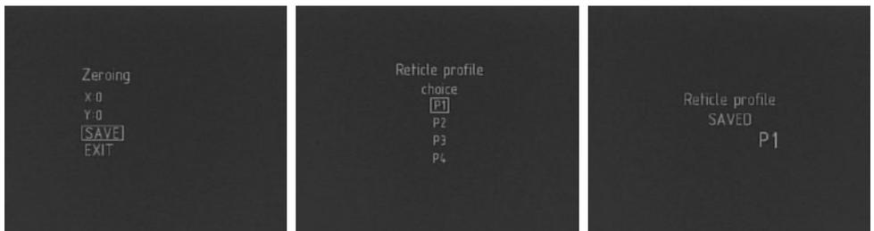
Using buttons A and B select the profile number and press and hold (more than 2 sec.) button M to save the zeroing results, and the display will show the message confirming the profile is saved.
