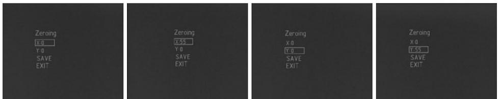
Fire 3-4 testing shots. Specify the shooting accuracy and the mean point of impact (MPI). If MPI deviates more than by the permitted value, re-enter the corrections.
